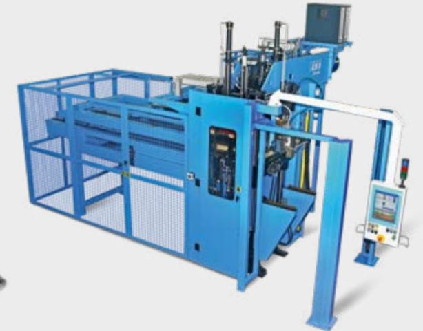
**+ FULLY-AUTOMATIC PRODUCTION CELL FOR THE PRODUCTION OF FUEL CELL SEALS**
