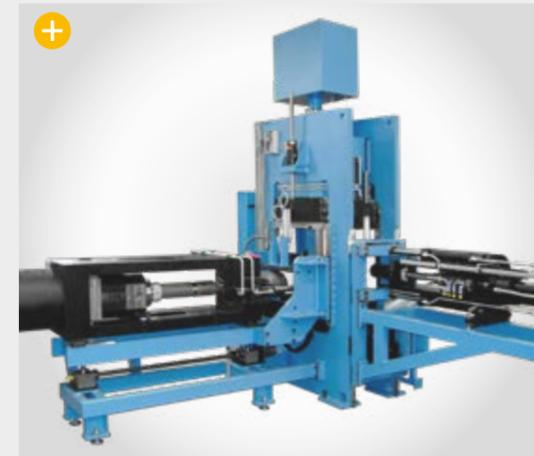
Downstroking press with two horizontally arranged injection units
