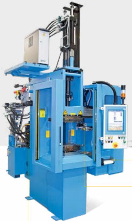
**+ VERTICAL ELASTOMER INJECTION MOULDING MACHINE**
