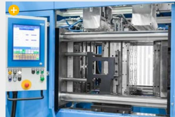
Brush modules for automated part removal and mould cleaning
