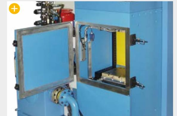
Easy access to the vacuum chamber for maintenance and mould loading
