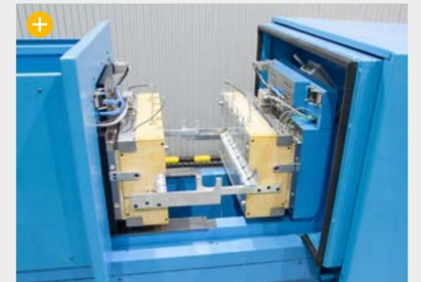
Horizontal C-frame machine for the production of isolators of liquid silicone
