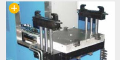
Quick latch system on separator and heating platen
