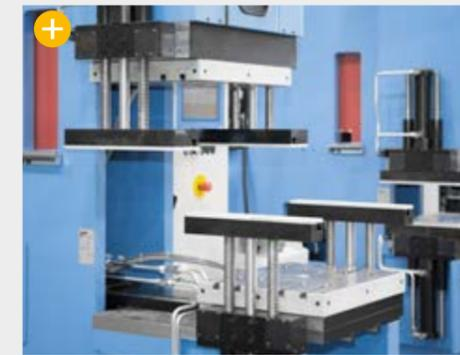
Demoulding with sliding table and separator
