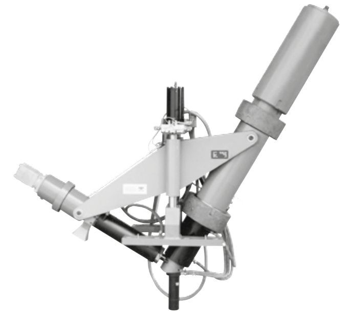
Milestone of its day The Y-shaped design of the injection unit was considered to be the state-of-the-art in the 1970s.
