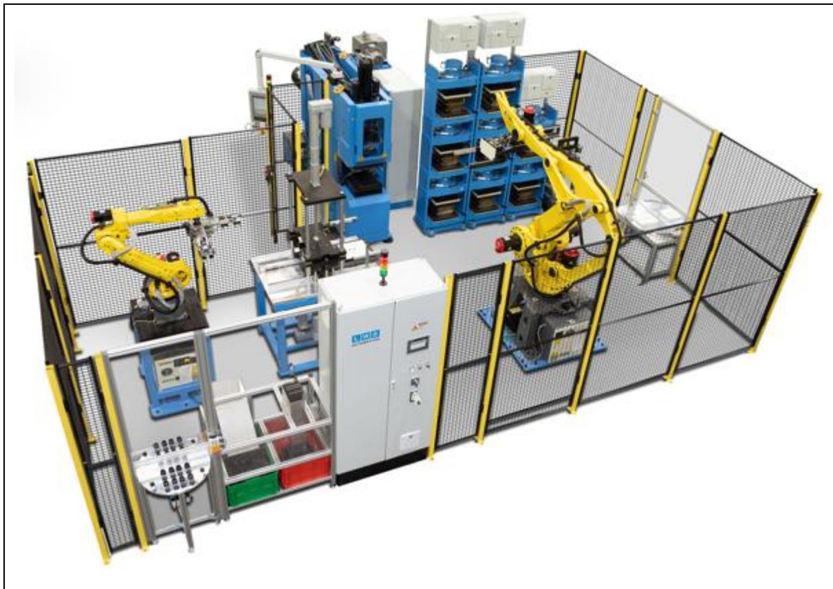
Fig.1: Configuration example of the modular LWB-multi-station-injection molding system
