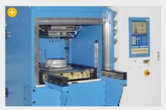
VP clamping unit in combination with a sliding table
