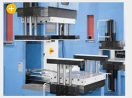
Demoulding with sliding table and separator
