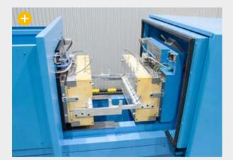
Horizontal C-frame machine for the production of isolators of liquid silicone
