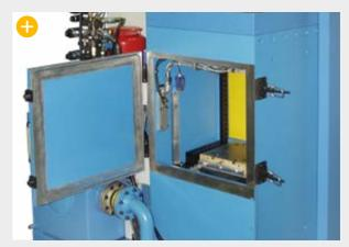
Easy access to the vacuum chamber for maintenance and mould loading
