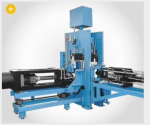
Downstroking press with two horizontally arranged injection units
